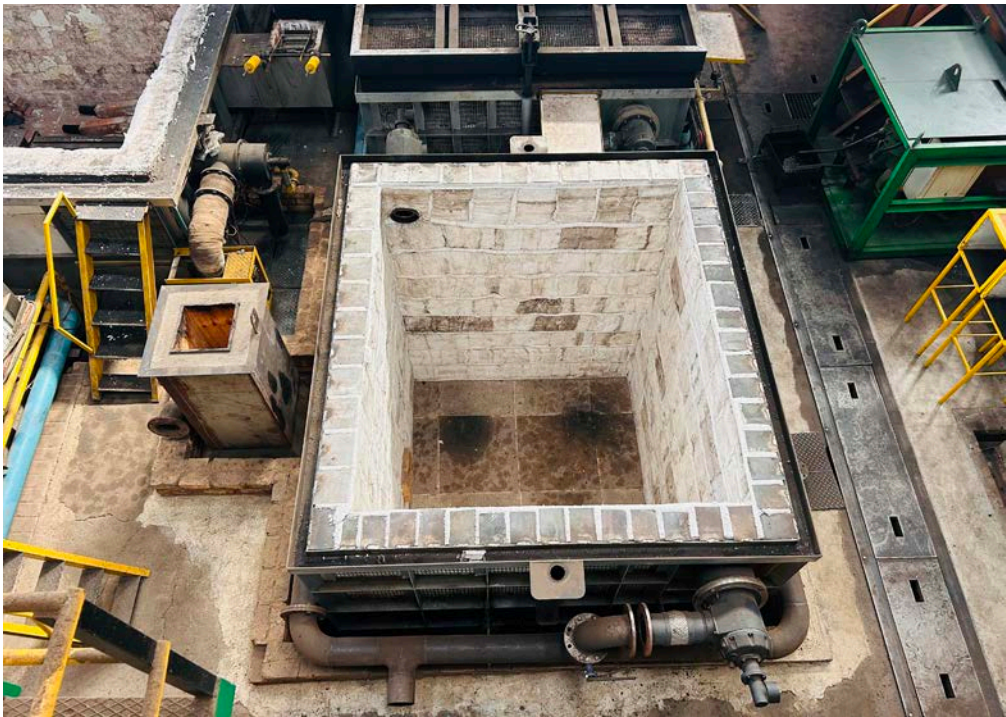
A brand-new pit furnace with recuperative burners
