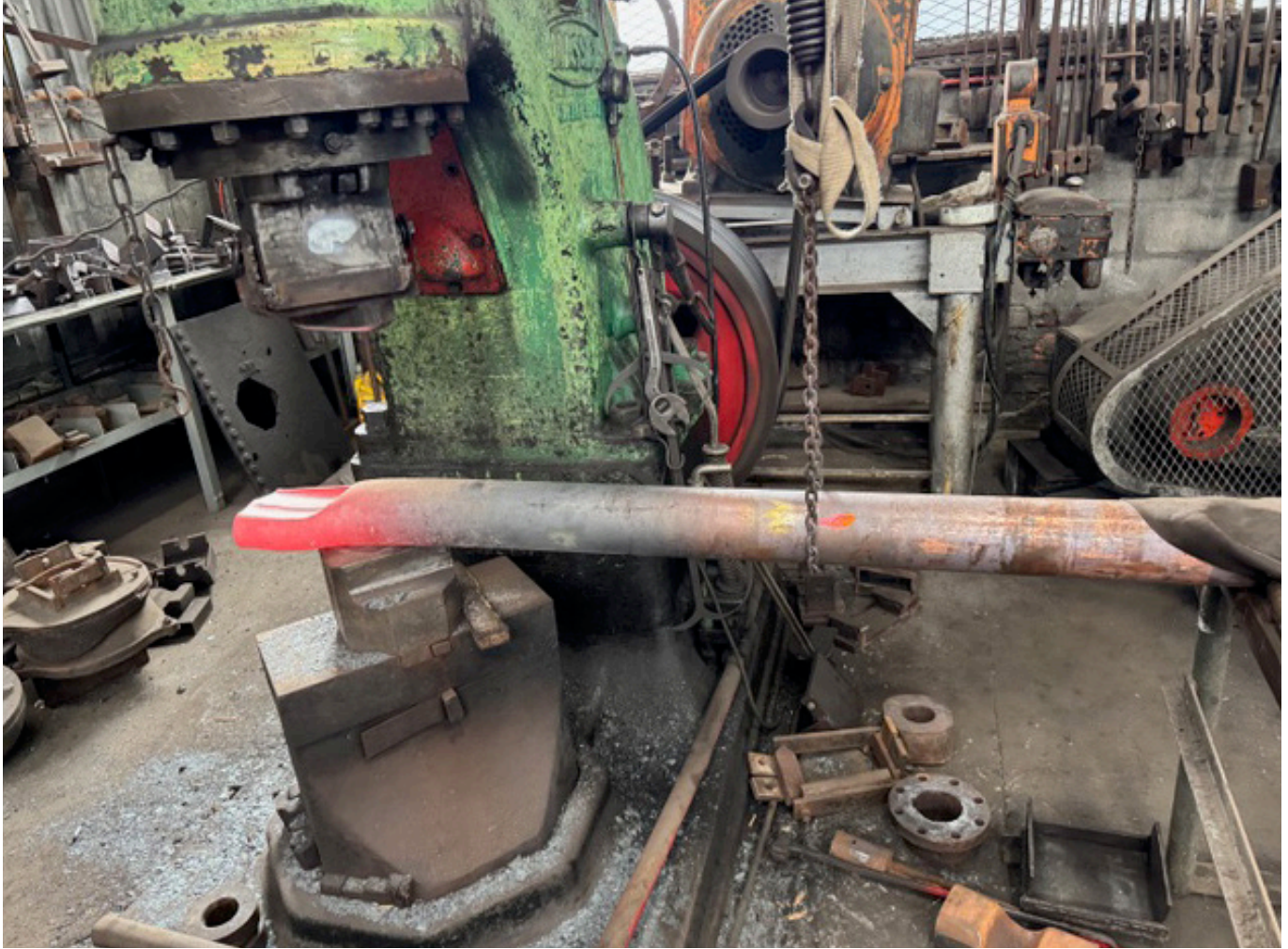
Large solid piece of copper in process on a power hammer – becoming a solid copper chaise
