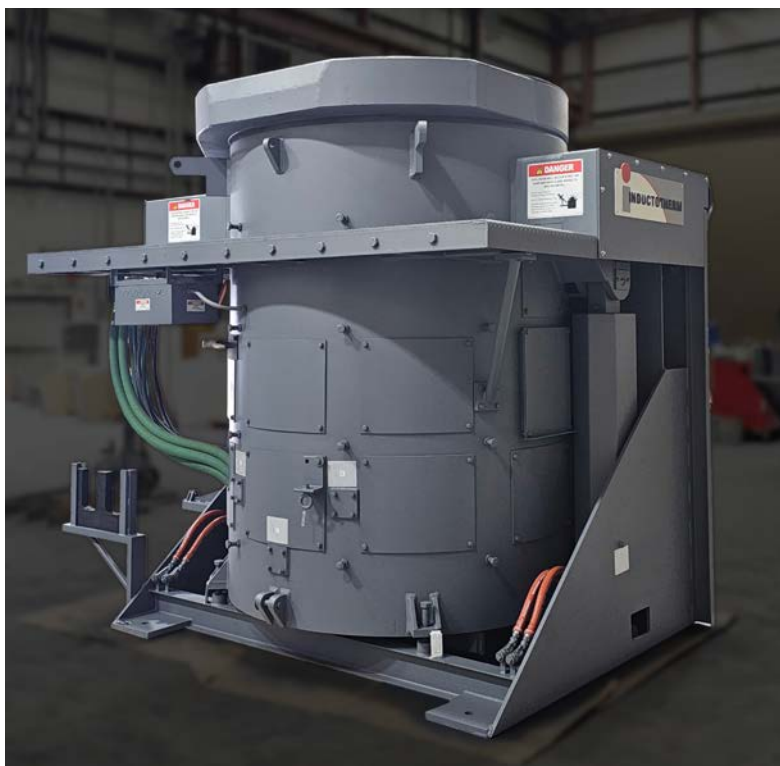
Inductotherm's five-ton, heavy steel shell was an ideal choice for Pier Foundry's output needs, due to its durability and reliability
