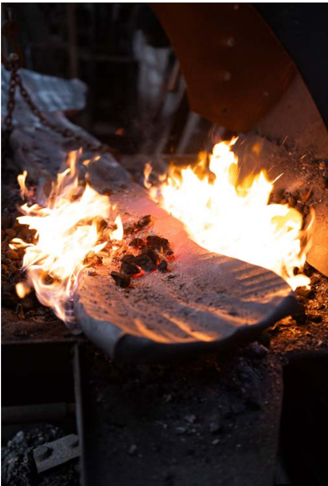
Before and during the shaping process, metal is first heated in a fire in a forge before it becomes soft and easier to manipulate. Once hot, the metal is transferred to an anvil or to a power hammer where it can be shaped using various tools
